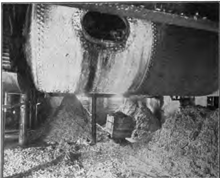
FIG. 135.—A boiler in which 12,000 pounds of rags are boiled at one time. (Courtesy of B. D. Rising Paper Co.)
